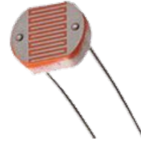
CDS Cell (light-sensitive resistor)
